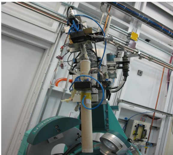
Figure 1.2 Psi-8 diffractometer detector arm with analyser setup.
